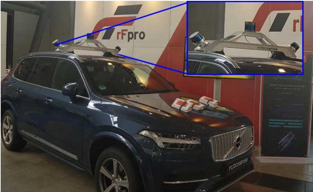
LIDAR(Laser Lader = Light Detection and Ranging)
