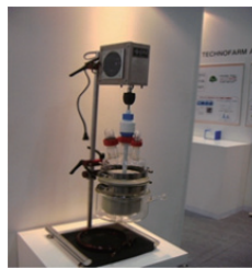
Filtering vessel using pressure for particles filtration(Powder system)
